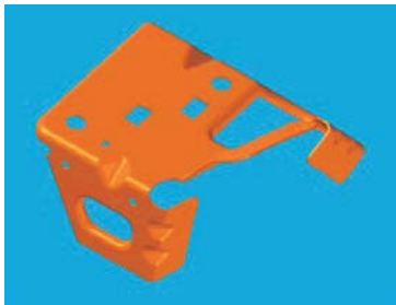
CAD model of bracket in Unigraphics
