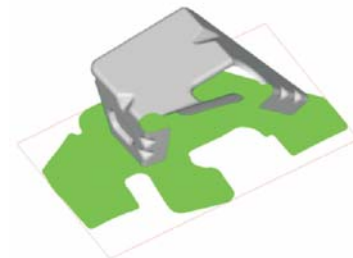
Part and blank as produced in FASTBLANK
