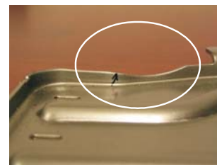
Washed out area is indicated by black arrow
