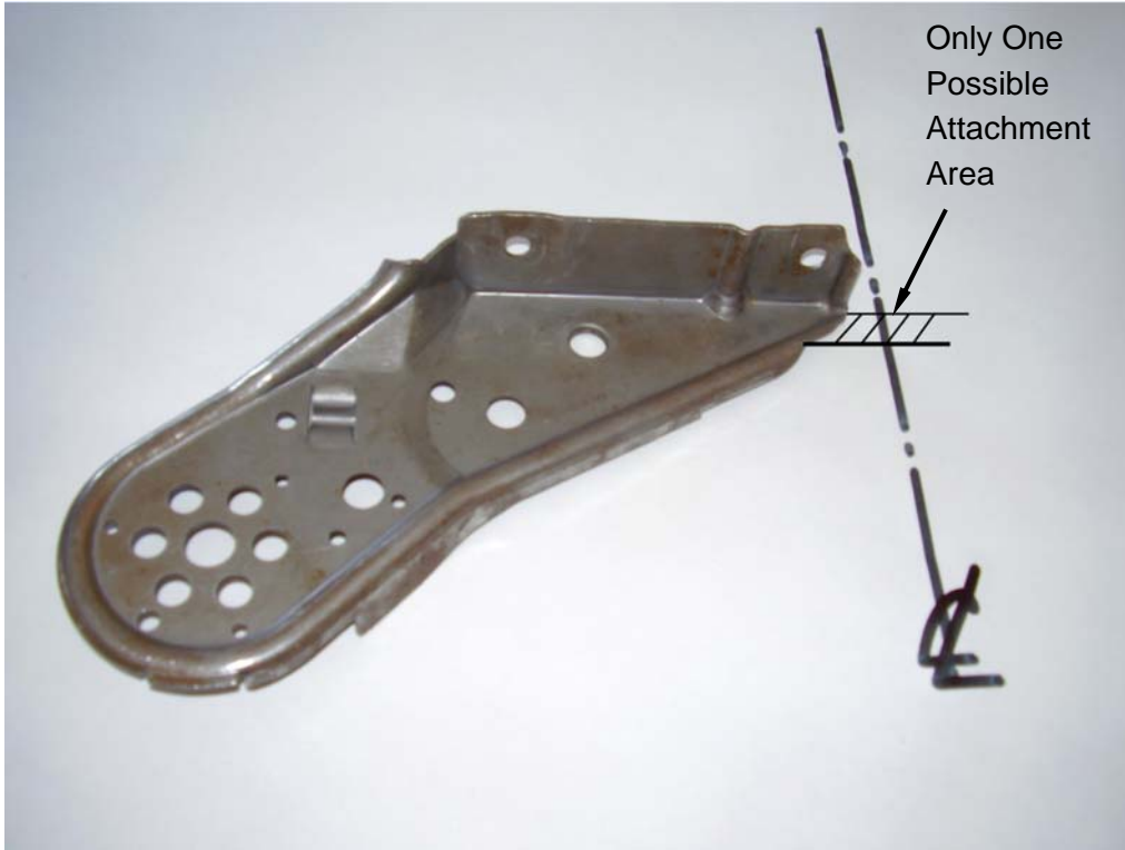
Figure 1-3. Part with Complex Geometry Resulting in a Difficult Attachment
